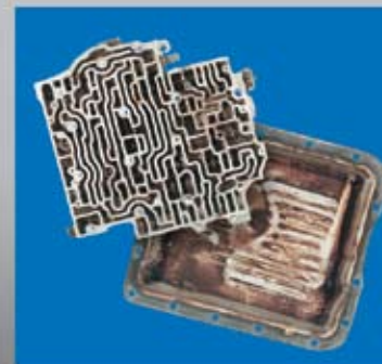
Transmission With Deposits
